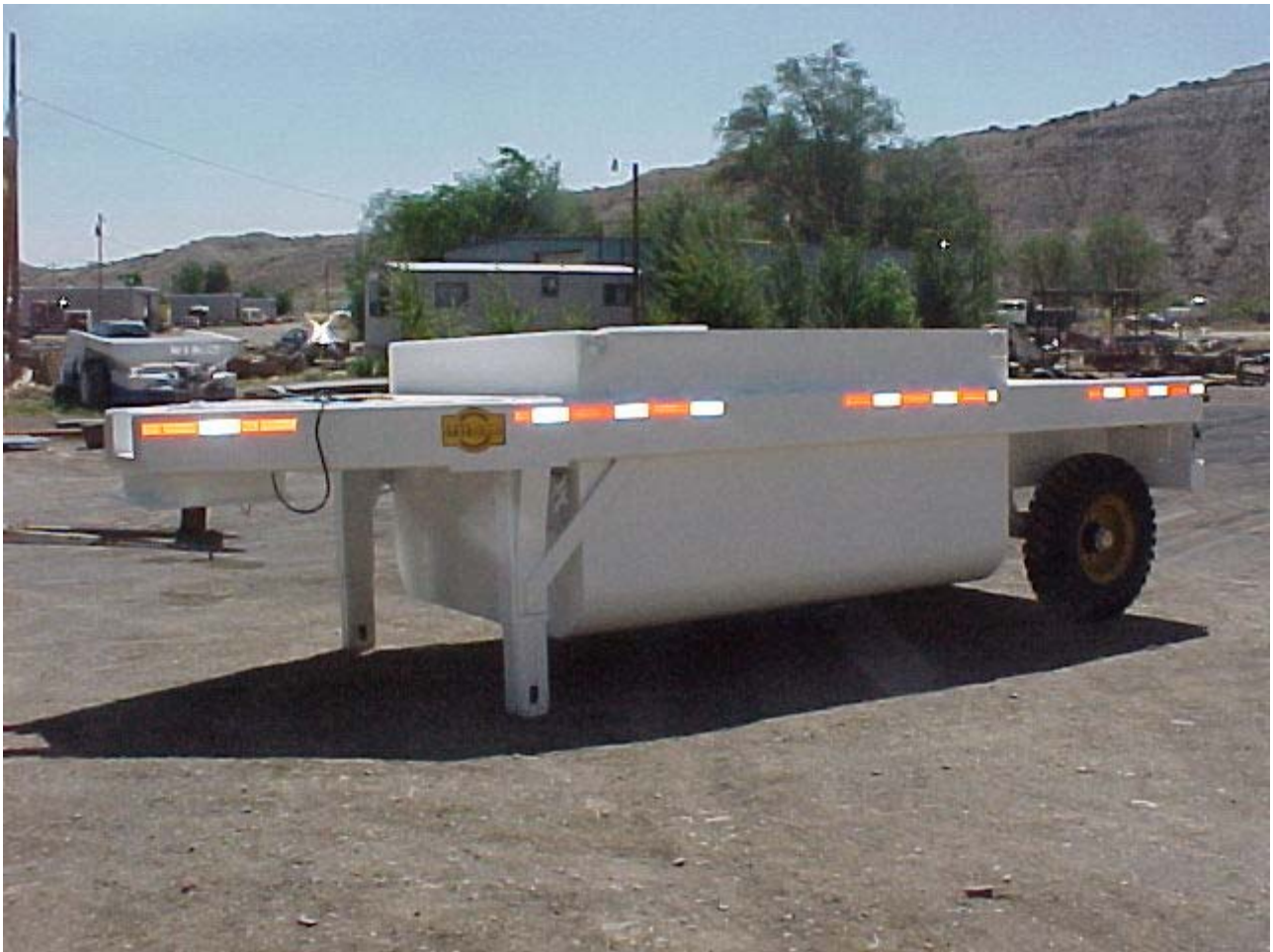
General arrangement of water wagon # 20254
